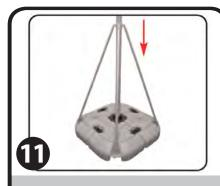
Slide the telescopic pole through the hole in the pole stay set.
