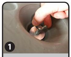
Place one spring into one of the two indentations on the top of the base and from the underside thread a washer then a finger screw onto the bolt until finger tight.
