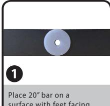
Place 20" bar on a surface with feet facing downwards. Place spacer on top, aligning spacer hole with center hole of the bar.
